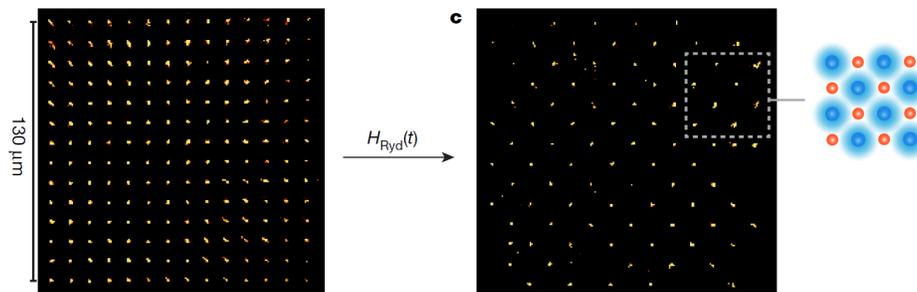
**Fig. 1:** Preparation of the antiferromagnetic ground state of the Ising model in a 196-atom square array [3].
